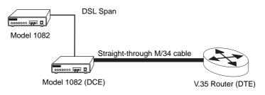
Figure 6. Connecting the Model 1082 to a V.35 serial DTE
